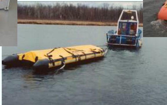
FLOATING STORAGE TANKS
